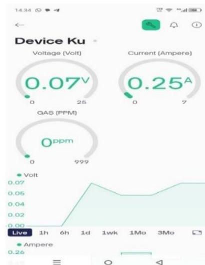
Figure 12. Blynk display shows the robot is on standby and has not detected the smell of butane gas
