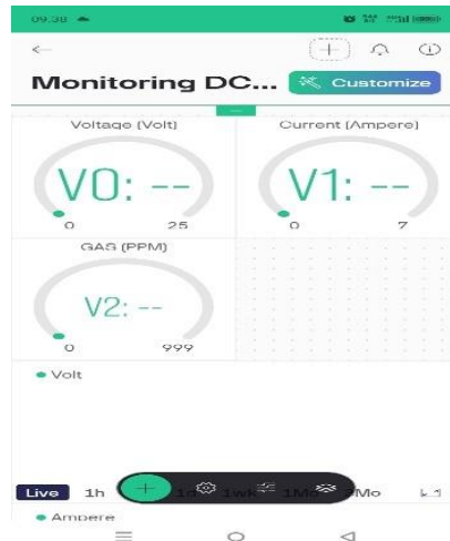
Figure 4. Initial design of the IoT display in the Blynk application
