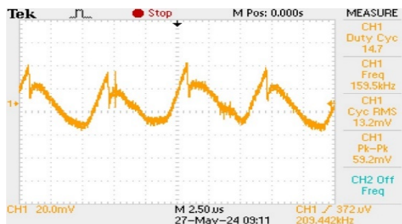
Gambar 5. Sampling Frekuensi Output PWM Baterai 12V 5ah K p =2, K i =5, K d =1
