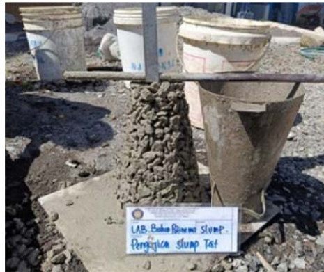
Gambar 2. Sample Slump Test Results
