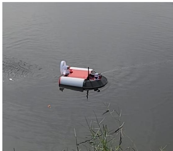
Figure 6. Hovercraft control distance test and spray
